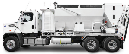
2. MOBILE BATCHING UNIT
